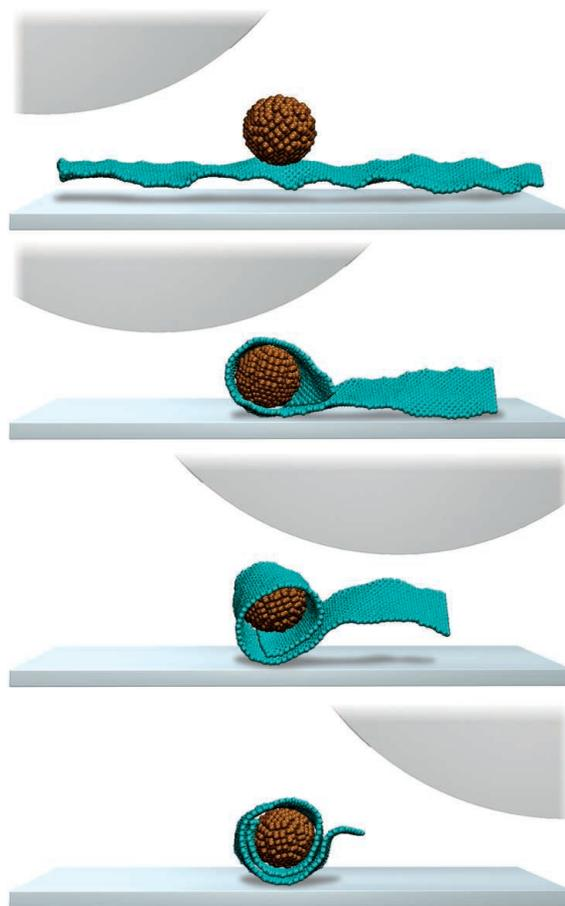
**Squeeze wrap.** Berman *et al.* found that huge reductions in macroscopic friction (“superlubricity”) were achieved where nanodiamonds slid against graphene. The nanodiamonds bonded to graphene nanoplatelets and became wrapped in them, allowing them to slide easily through incommensurate surface effects.
